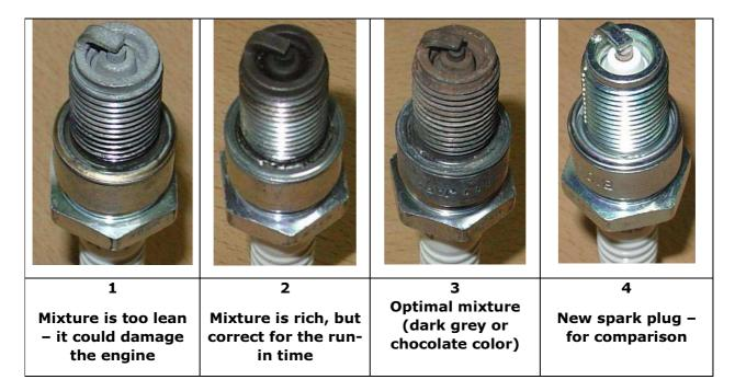
During the run-in time a wet and tarry spark plug is a good sign because it means that the mixture is rich. Petrol in a two-stroke engine is not only a fuel, but also a heat conductor, which is emitted excessively during the run-in. During the run-in time, we advise you to error on the side of caution and use a rich mixture at the expense of slightly weaker engine performance.
